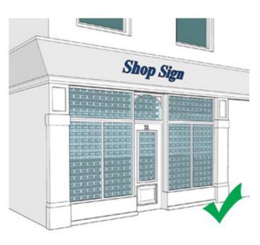
Security shutters should not be used externally, but instead behind internal lattice grilles, or preferably, laminated glass
