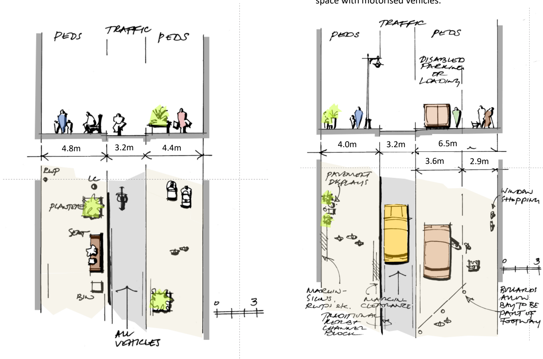
Figure 7.5 and 7.6. Sections through High Street, showing wider footways, furniture zones and narrow carriageway with cyclists sharing space with motorised vehicles.
