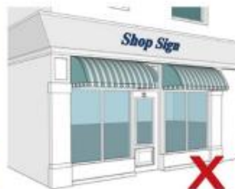
Non-retractable Dutch blinds should not be used
